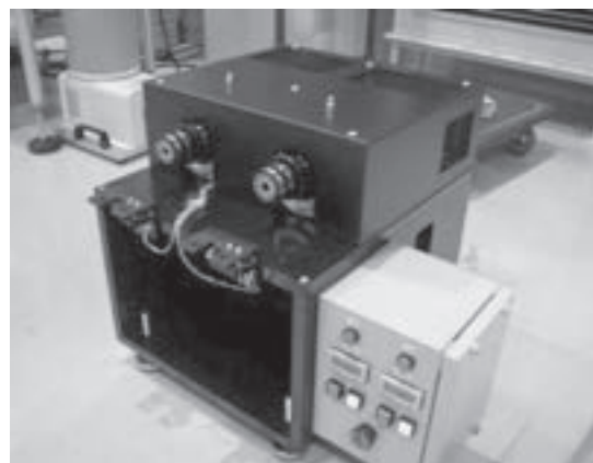
Fig.6 Cantilever type fatigue machine.
